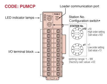
**LEDindicator** Three LED lamps indicate the following operational conditions
